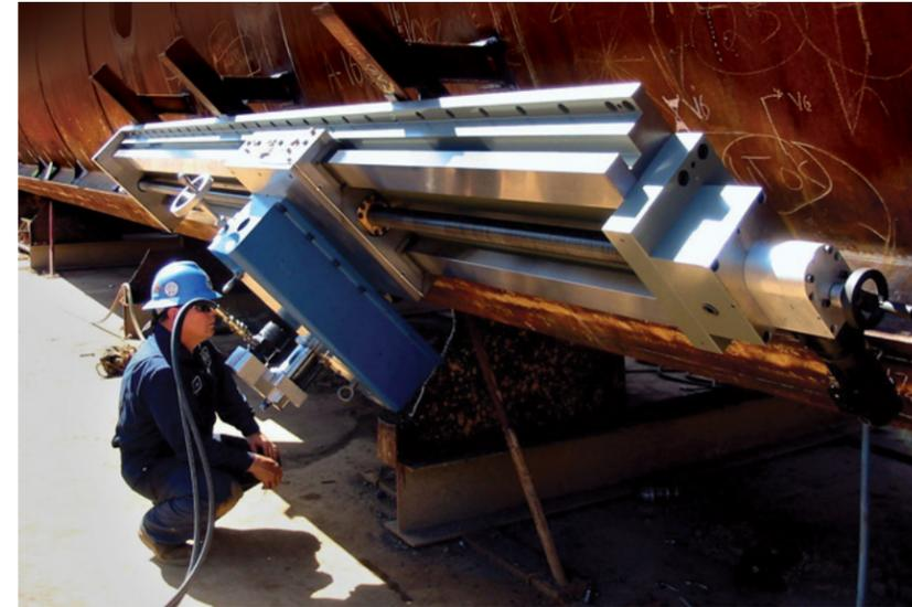
TEAM has one of the largest in-stock supplies of field machining equipment in the world. Additionally, we custom design and fabricate specialty equipment to handle a number of challenges. All machines are pneumatically and hydraulically powered for use in plant environments where intrinsically safe operations are mandatory.
