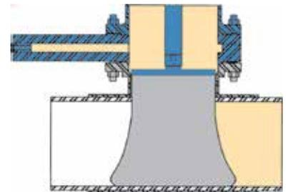
Top Right: Cylindrical rubber line stop machine assembled with valve and fitting. Cylindrical rubber stopper is in Line Stop position. Pressures to 100 psi (7 bar).
