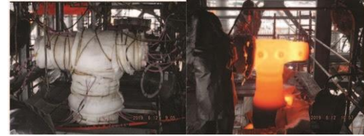
Figure 2. The effects of electrical resistance heat treating on a stainless steel header being annealed. Left: wrapped; right: unwrapped.
