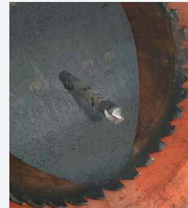
36" Hot / Wet Tap cutter, coupon and pilot drill
